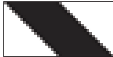
This enlargement of a bitmap image clearly shows how a bitmap image is made up of little blocks.
